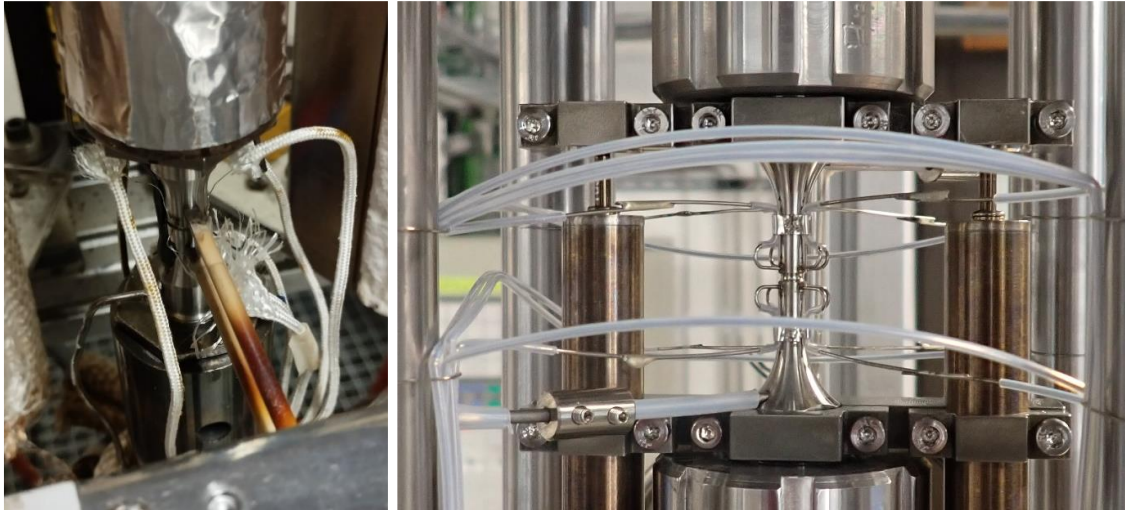
Figure 4.28. DCPD set-up in air (left) and PWR (right) environment.
